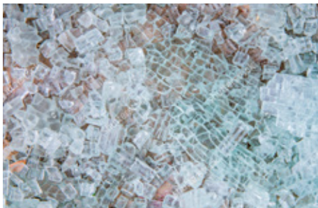
If toughened glass breaks, it shatters into relatively harmless small particles
